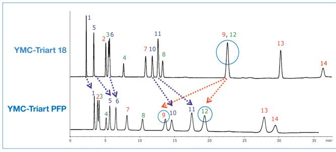
Figure 2: Separation of catecholamines using YMC-Triart C18 (top) compared to YMC-Triart PFP (bottom).
