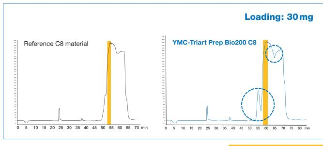
However, on increasing the loading the picture changes. For a loading of 30 mg, the YMC-Triart Prep Bio200 C8 phase still shows a good separation whereas the reference C8 material shows strong overloading effects.
