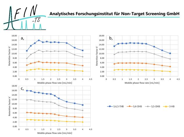
Figure 2: Retention dependency of mobile phase flow rate at different back pressure levels (a, 100 bar; b, 150 bar; c, 200 bar back pressure)
