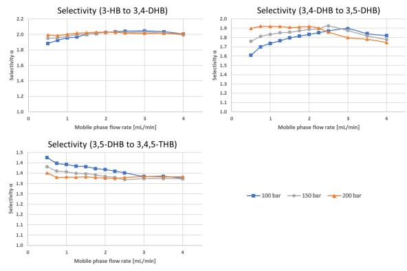
Figure 3: Selectivity dependency of mobile phase flow rate and back pressure level
