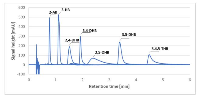
*Figure 1: Chromatogram of 7 of the 17 compounds, which were tested under isocratic conditions. The chromatographic conditions were not optimized.*
