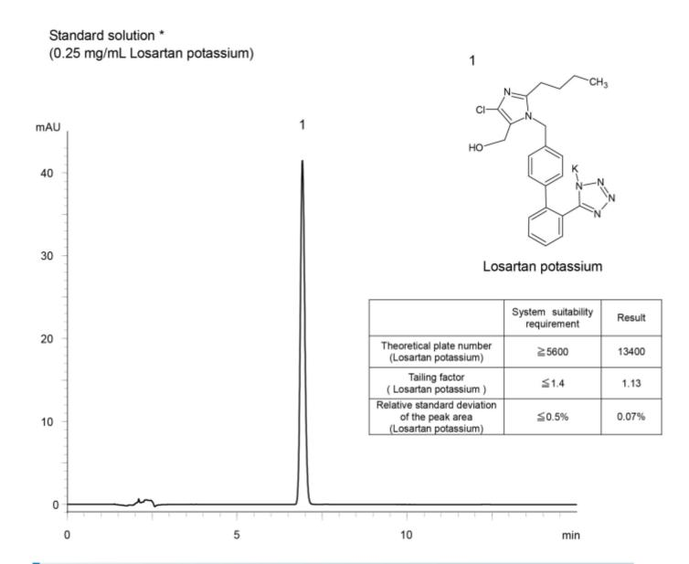
Column : YMC-Triart C18 (5 µm, 12 nm)
