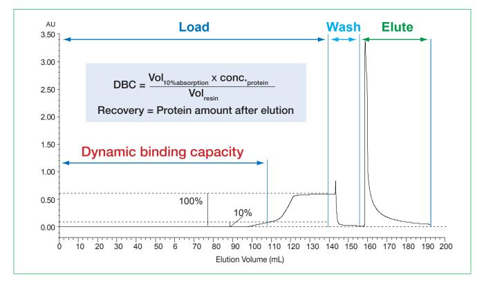
To determine the DBC, a protein solution with a defined concentration is pumped through the column and the proteins bind to the column. The solution is pumped until a flow through of the protein is detected and saturation is reached. Afterwards, the amount of protein that was pumped through the column until a protein breakthrough at 10% of the saturation is calculated. This value for the binding capacity can be normalised on the resin volume: **DBC = mg bound protein/mL resin**
