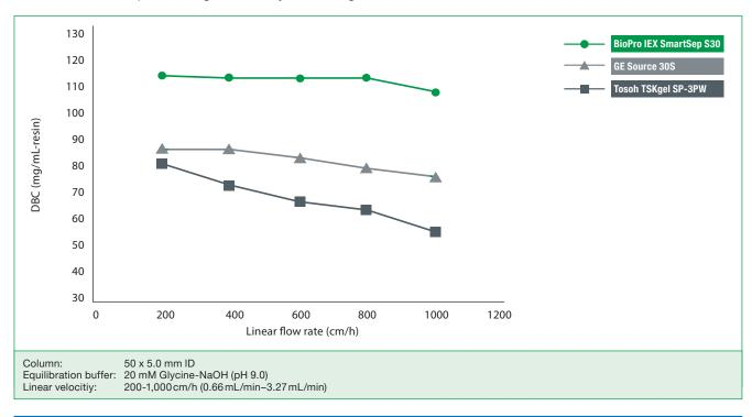
High flow rates further improve the productivity of the purification because they additionally increase the throughput. Therefore, a combination of high loadings and high velocities are ideal for efficient processing. BioPro IEX combines both – high loadability and high flow rates.
