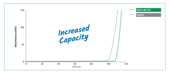
BioPro IEX shows a later breakthrough of the IgG compared to the alternative material, so more of the antibody could be bound to the resin before the breakthrough was reached. Therefore, BioPro IEX has a higher DBC for the monoclonal antibody.
