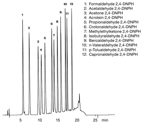
Column: YMC-Pack C<sub>4</sub> (5 μm, 12 nm) 150 x 4.6 mm ID
