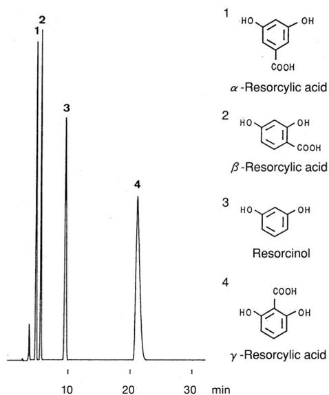
Column: YMC-Pack C<sub>8</sub> (Octyl) (5  $\mu$ m, 12 nm) 150 x 4.6 mm ID
