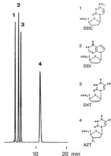
Column: YMC-Pack C<sub>4</sub> (5 μm, 12 nm) 150 x 4.6 mm ID
