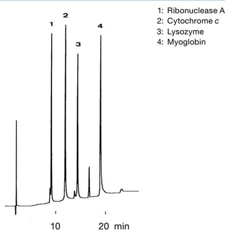
Column: YMC-Pack C<sub>4</sub> (5 μm, 30 nm) 150 x 4.6 mm ID
