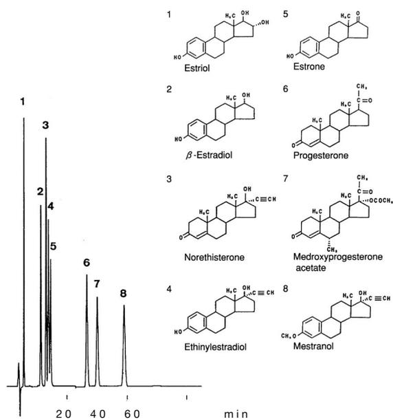
Column: YMC-Pack C<sub>8</sub> (Octyl) (5  $\mu$ m, 12 nm) 250 x 4.6 mm ID
